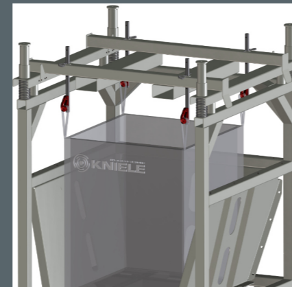
Traverse with spring tension
